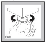
Accurate levelling prevents vibration, noise and displacement of the machine during operation. Never place cardboard, wood or similar materials under the machine to compensate for any unevenness in the floor. After having levelled the machine, tighten the lock nuts.
